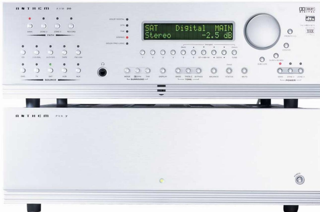
The major difference between THX Cinema and THX Surround EX is that the latter requires two more speakers, placed in the rear, which are designed to enhance the sense of ambient envelopment when used with appropriately encoded program material. The Anthem amplifier line already had a 5-channel amplifier suitable for Dolby Digital/DTS/THX Cinema; the new product, the Anthem PVA 7, is designed to accommodate the amplification requirements of THX Surround EX.
