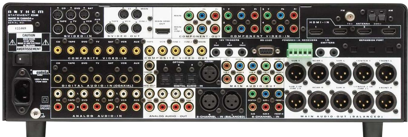
Currently, the D2's input EDID information relays that it can support up to 96/24 for input audio resolution. It also does all of its post-processing (bass management, time alignment, PL-IIx, THX, etc.) at that level then up-samples to 192/24.
