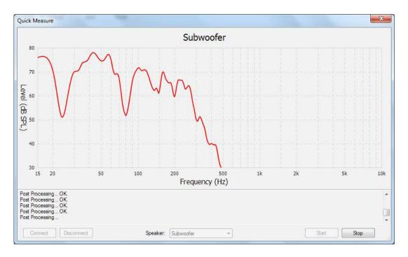
They can almost always be cured by repositioning speakers and repeating the measurement:
