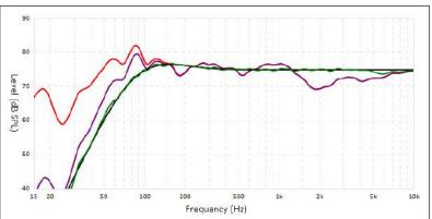
The red curves represent the in-room response before correction, as an average from five measurement positions, whereas the green ones show response with equalization applied. In this case a subwoofer and bass management are also in use. In the subwoofer graph, which is on the left, the difference between the level of the red and purple curves shows the amount of room gain.
