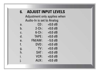
If a source that is set to Analog-DSP is playing while you adjust the Input Level, you will notice a vertical bar graph to the left of the dB setting. With the On-Screen display, if this Bar Graph changes from green to pink, you have gone into an overload condition. Reduce the level until the bar graph changes back to green.
