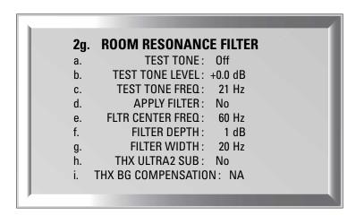
Rooms often have a single prominent resonance peak which can make bass sound boomy, even with the finest subwoofer. The AVM 20 has a proprietary set of low frequency test tones that allow you to find and easily remove that resonance peak.
