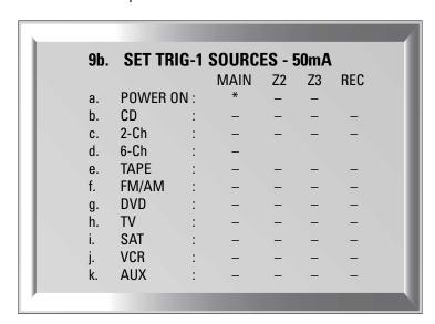
Under each of the four AVM 20 Paths, MAIN, ZONE2 (**Z2**), ZONE3 (**Z3**), and RECORD (**REC**), notice that there are 40 available Sources (40 dashes) that could be used to activate the trigger. After highlighting POWER ON or a Source, press **SELECT** and use the ◀ ▶ buttons to move from one Path to another, and then to set the trigger to activate, use the ▲ ▼ buttons to change the '−' to a '\*'.
