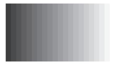
Black level is one step below the pattern's darkest bar and full level is one step beyond the brightest bar.
