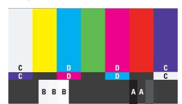
Color Bars is the SMPTE test pattern, with bars at 75% saturation:
